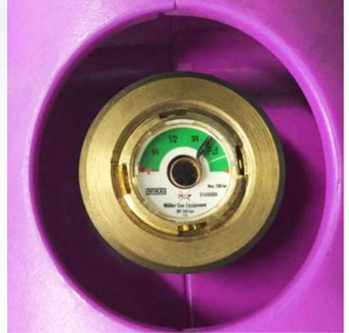
4. Verify that the contents pressure indicator (on the side of the handle) is showing the gas contents left in the cylinder.
