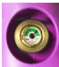
4. Verify that the contents pressure indicator (on the side of the handle) is showing the gas contents left in the cylinder.
